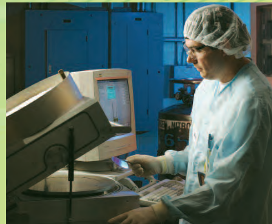
Graduate student Chris Siebert is studying optoelectronic devices. The plasma-enhanced chemical vapor deposition system he is using here deposits an optical antireflection coating on the wafer.
