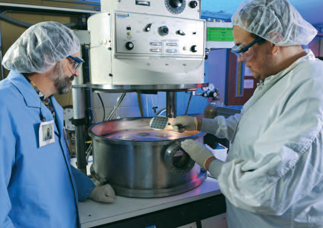
Gregory Snider, left, professor of electrical engineering, and Aaron Prager, graduate research assistant, are loading a wafer into a sputter deposition system, which will coat the wafer with metal for forming transistors on the electrical interconnections between transistors.
